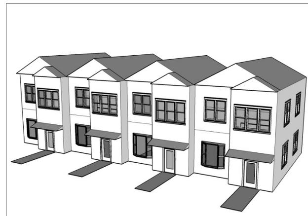
33 **(2)** Wall offsets shall have a minimum depth of two feet.
