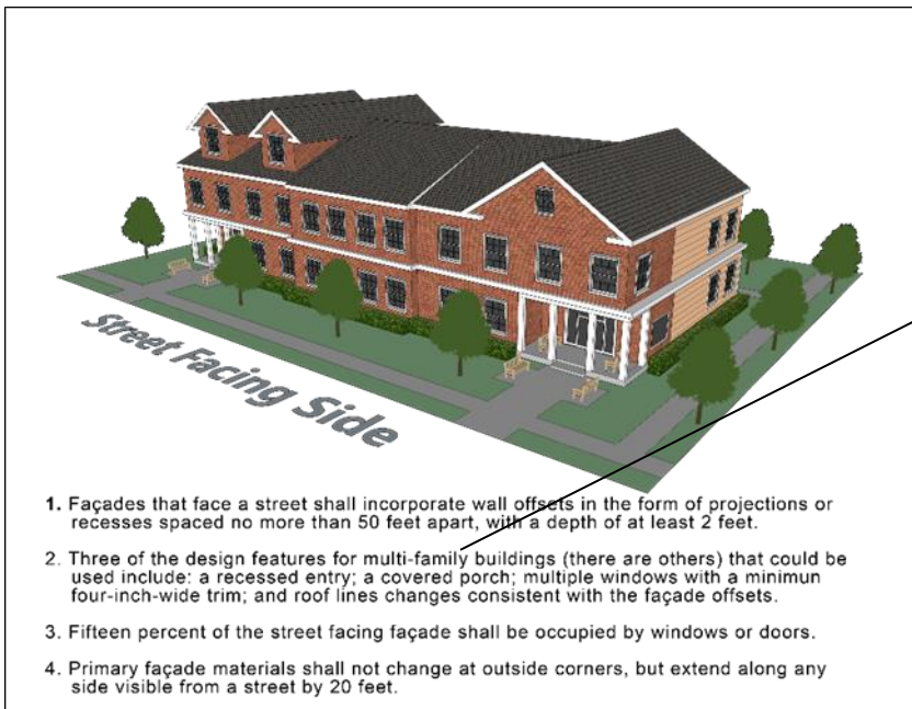
11 Figure 27-6903(h): Example of Building Façade, Roof, Fenestration/Transparency and 12 Materials Requirements for Multifamily Building
