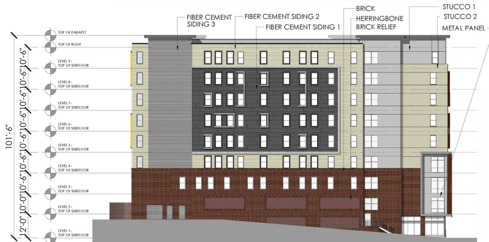
Figure 3: Building 1 West Elevation
