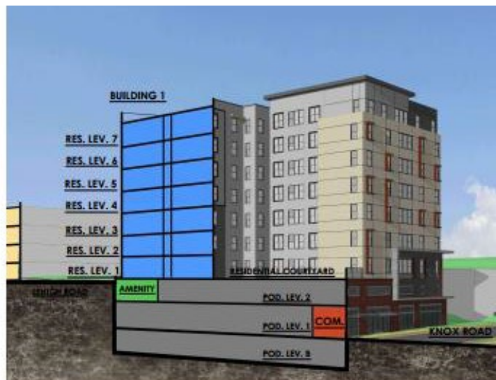
Figure 16: Site Diagram Showing Parking Garage Placement
