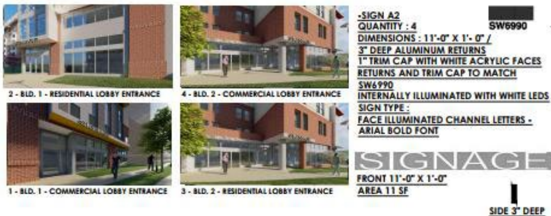
Figure 14: Sign above residential and commercial entrances at Buildings 1 and 2
