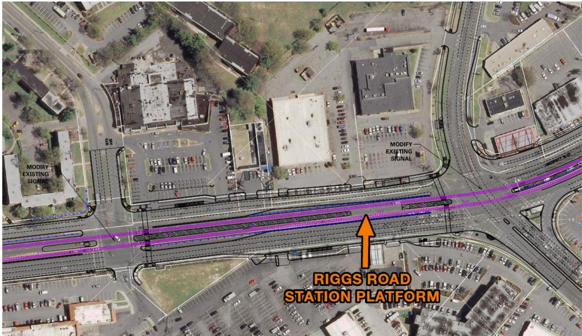
The above image also shows that the station will be in the median of the road, maintaining access to the side from University Boulevard.
