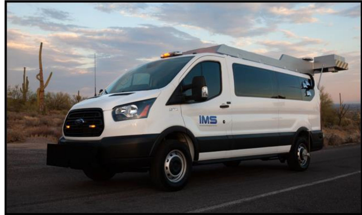
Pavement Survey Vehicle
