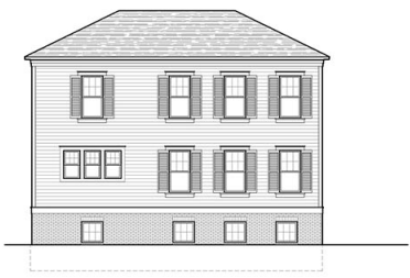
8 SIDE ELEVATION - NO PORCH - SIDING A2.5 1/8" = 1'-0"
