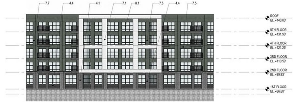
3 COURTYARD ELEVATION - NORTH SCALE: 1/16" = 1'-0"
