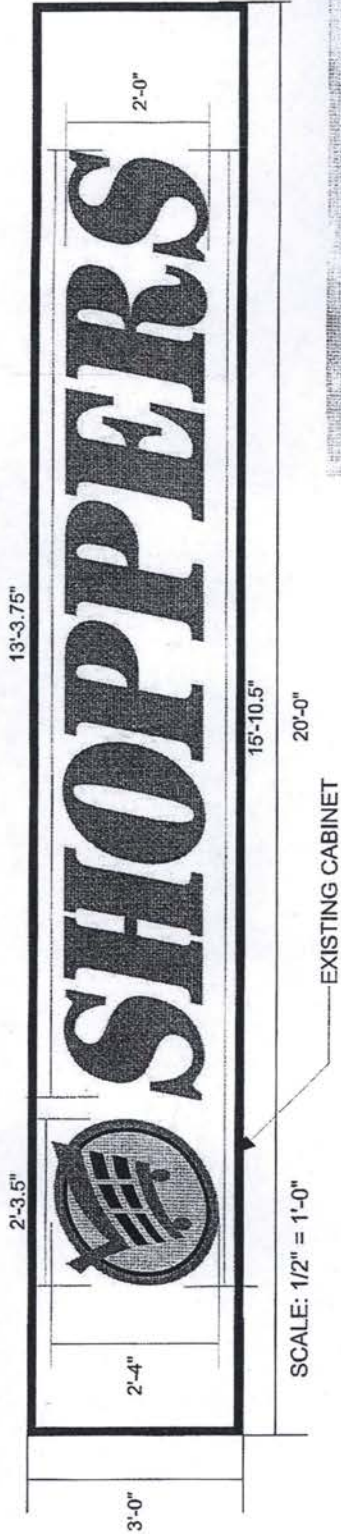
REAR PYLON REPLACEMENT FACE ABOVE SUBWAY SIGN
