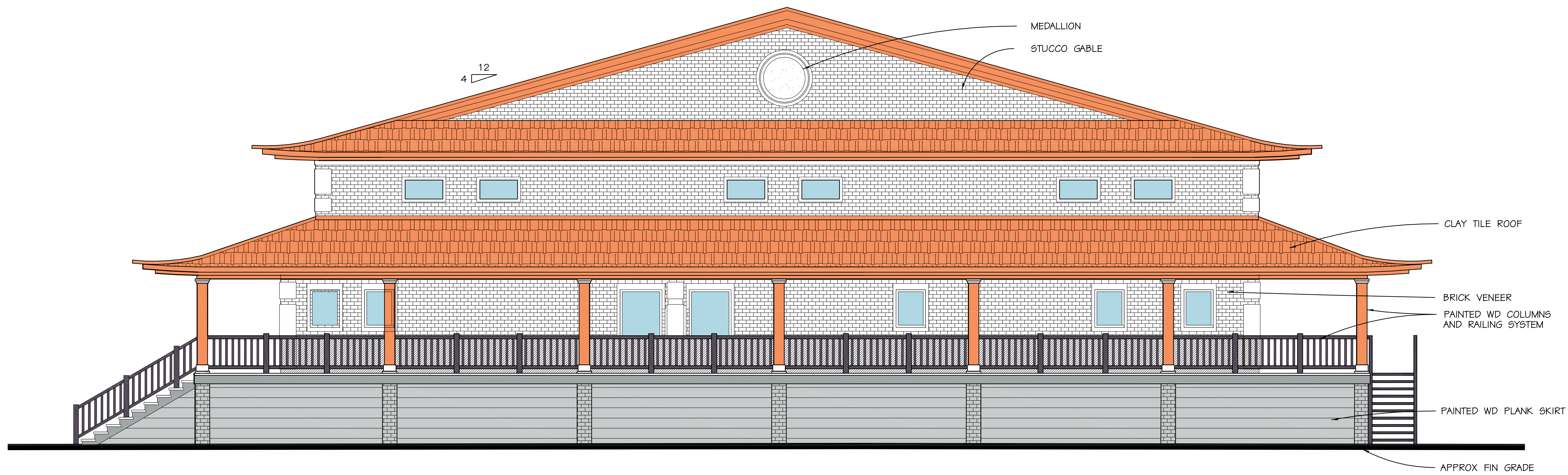
B EXTERIOR ELEVATION @ LEFT SIDE (NORTH WEST) 1/4" = 1'-0"
