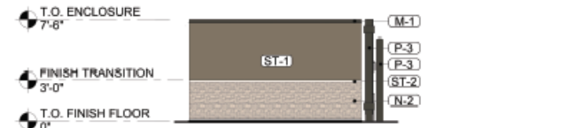
3 SIDE DUMPSTER ENCL. ELEVATION RBE-2 SCALE: 1/4" = 1'-0"
