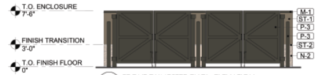
5 FRONT DUMPSTER ENCL. ELEVATION RBE-2 SCALE: 1/4" = 1'-0"
