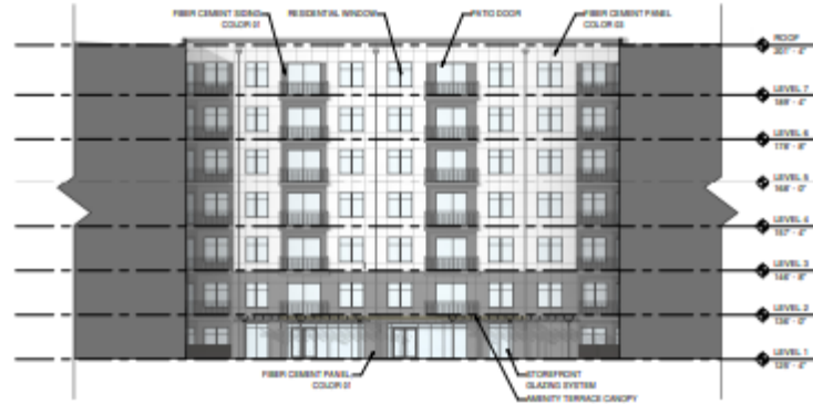
F7 NORTH COURTYARD - WEST ELEVATION
