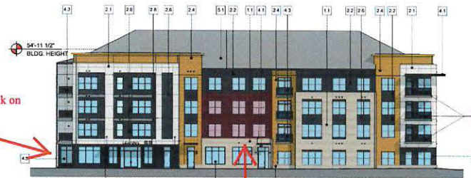
This section will be changed to Brick - Tag 1,2. 3 BUILDING 1000 SOUTH ELEVATION 1/16" = 1'-0"
