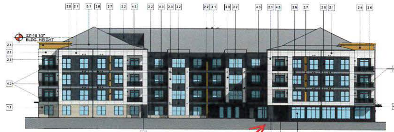
The entire 1st floor of this elevation is brick. Just a really dark color on the bottom floor that looks similar to the cementitious panel. 4 BUILDING 1000 WEST ELEVATION 1/16" = 1'-0"
