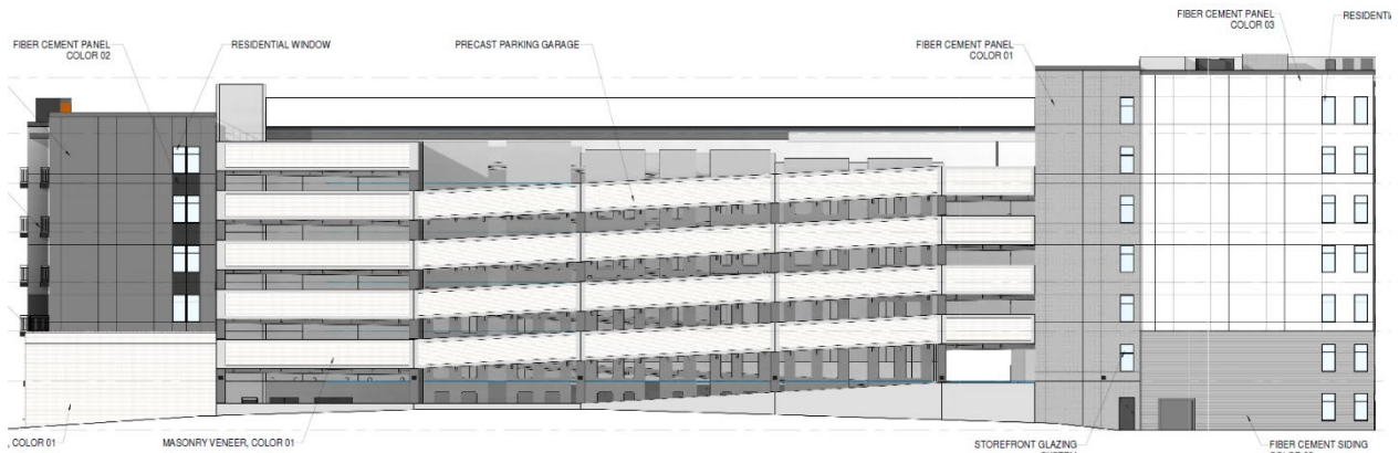
Figure 2: East Elevation Showing Structured Parking
