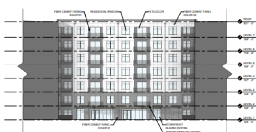
F7 NORTH COURTYARD - WEST ELEVATION
