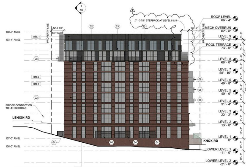
2 BUILDING ELEVATION - WEST 1/16" = 1'-0"
