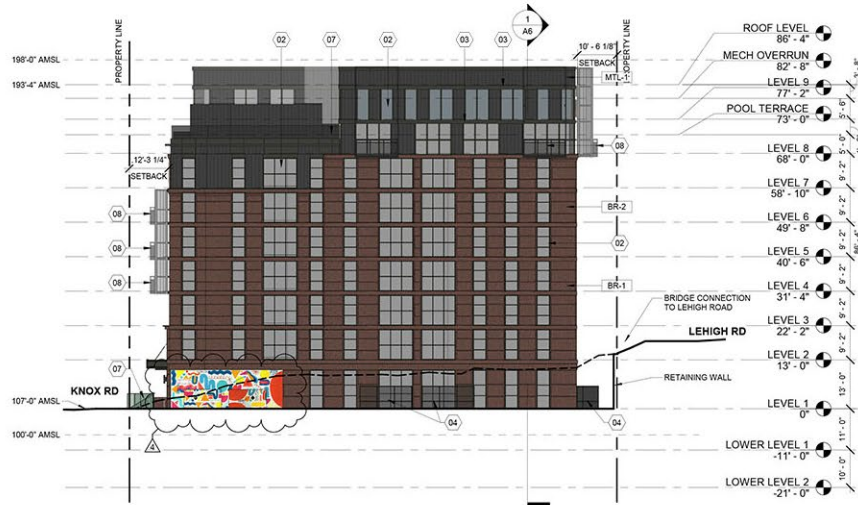
1 BUILDING ELEVATION - EAST 1/16" = 1'-0"
