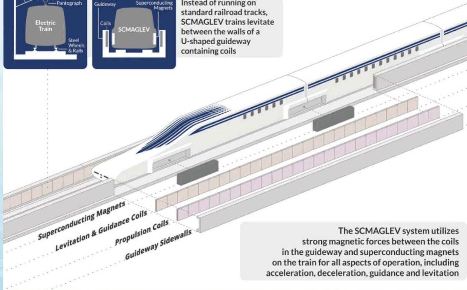
The SCMAGLEV system utilizes strong magnetic forces between the coils in the guideway and superconducting magnets on the train for all aspects of operation, including acceleration, deceleration, guidance and levitation
