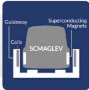
Instead of running on standard railroad tracks, SCMAGLEV trains levitate between the walls of a U-shaped guideway containing coils
