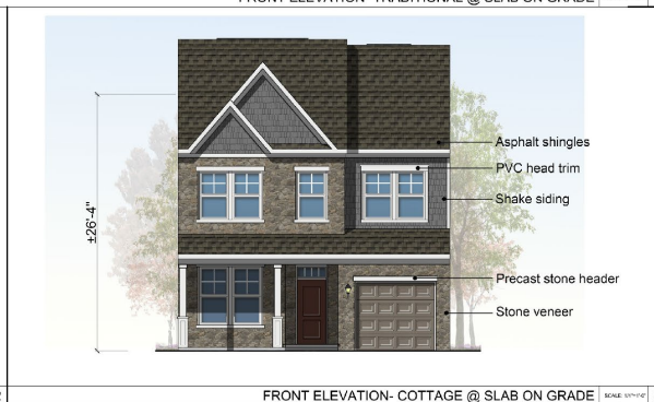
FRONT ELEVATION- COTTAGE @ SLAB ON GRADE | SCALE: 1/8"=1'-0" | 3
