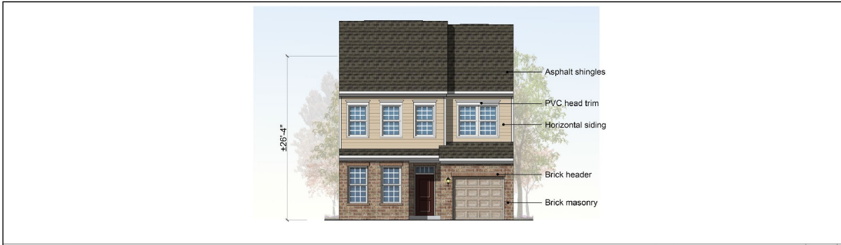
FRONT ELEVATION- TRADITIONAL @ SLAB ON GRADE | SCALE: 1/8"=1'-0" | 1
