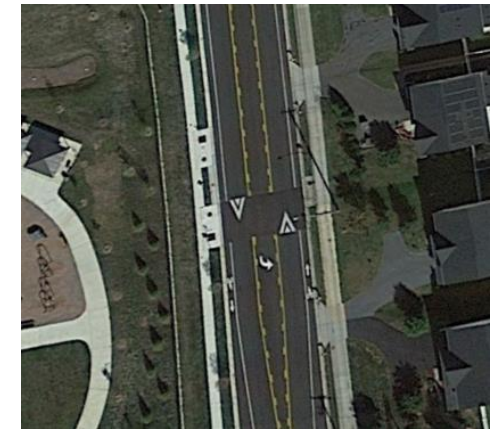
Speed Hump and Bike Lane
