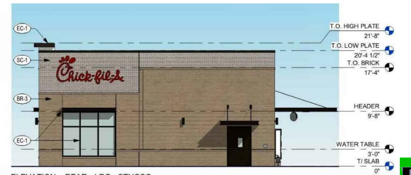
ELEVATION - REAR - LRG - STUCCO 1/8" = 1'-0"
