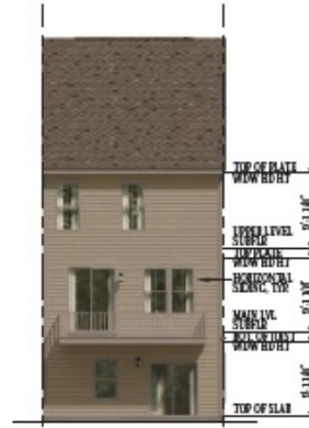
2 REAR ELEVATION SCALE 1/4"=1'-0" SHOWN W/ OPT. CANT'D DECK STANDARD REAR DOES NOT HAVE A DECK
