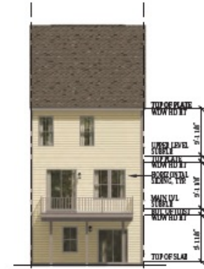
2 REAR ELEVATION SCALE 1/4"=1'-0" SHOWN W/ OPT. PORCHED DECK STANDARD REAR DOES NOT HAVE A DECK
