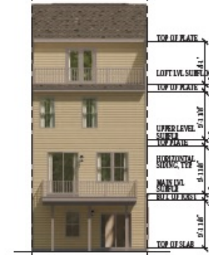
2 REAR ELEVATION SCALE 1/4"=1'-0" SHOWN W/ OPT. CANT'D DECK & OPT. LOFT TERRACE STANDARD REAR DOES NOT HAVE A DECK
