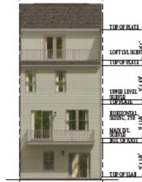
2 REAR ELEVATION SCALE 1/4"=1'-0" SHOWN W/ OPT. CANT'D DECK & OPT. LOFT TERRACE STANDARD REAR DOES NOT HAVE A DECK
