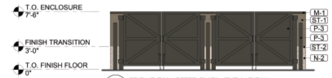
5 FRONT DUMPSTER ENCL. ELEVATION RBE-2 SCALE: 1/4" = 1'-0"
