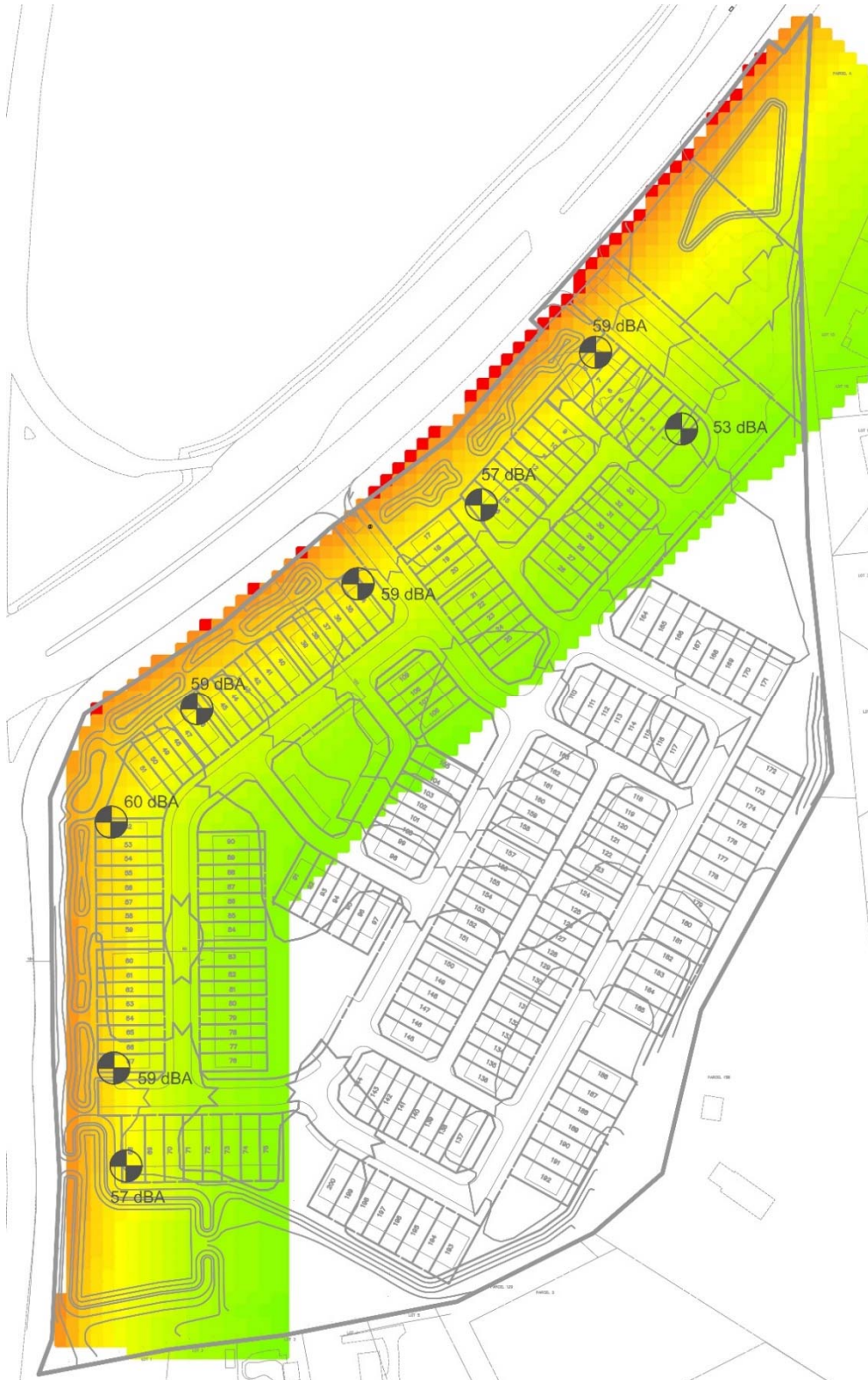
Figure 3. EXPECTED NOISE EXPOSURE from MD. RTES. 450 and 193 COMBINED outdoor day-night average sound levels ( L_{dn} ); ignoring shielding from proposed on-site structures; location-specific sound levels as per Table 2; color gradient denotes 50 dBA[ L_{dn} ] to 70 dBA[ L_{dn} ] noise exposure range
