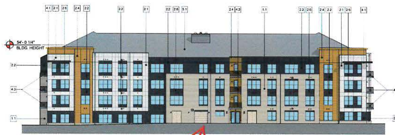
Three "Service" doors have been painted to match surrounding material colors. Garage door will be changed to double doors. 2 BUILDING 1000 EAST ELEVATION 1/16" = 1'-0"
