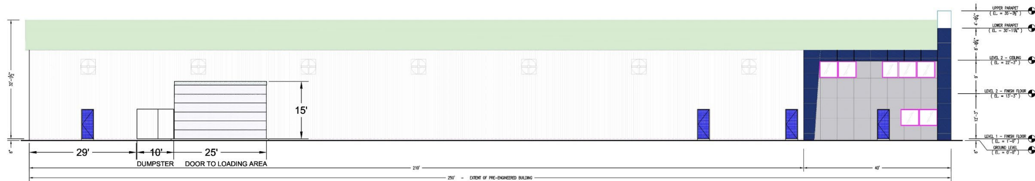
3 SIDE ELEVATION - SOUTH A1.0 3/32" = 1'-0"
