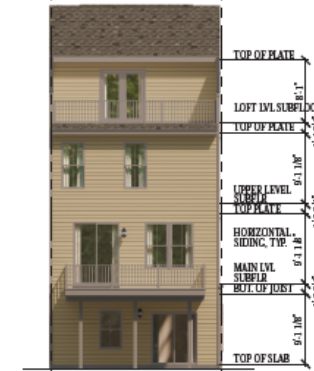
2 REAR ELEVATION SCALE 1/8"=1'-0" SHOWN W/ OPT. CANT'D DECK & OPT. LOFT/TERRACE STANDARD REAR DOES NOT HAVE A DECK
