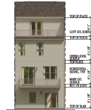
2 REAR ELEVATION SCALE 1/8"=1'-0" SHOWN W/ OPT. CANT'D DECK & OPT. LOFT/TERRACE STANDARD REAR DOES NOT HAVE A DECK
