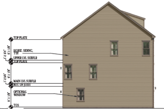
3 SIDE ELEVATION SCALE 1/8"=1'-0" SHOWN W/ ELEV. "M"
