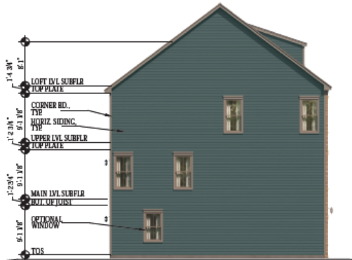
3 SIDE ELEVATION SCALE 1/8"=1'-0" SHOWN W/ ELEV. "M" & OPT. LOFT/TERRACE
