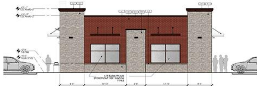
02 SIDE (NORTH-WEST) ELEVATION 3/16" = 1'-0"
