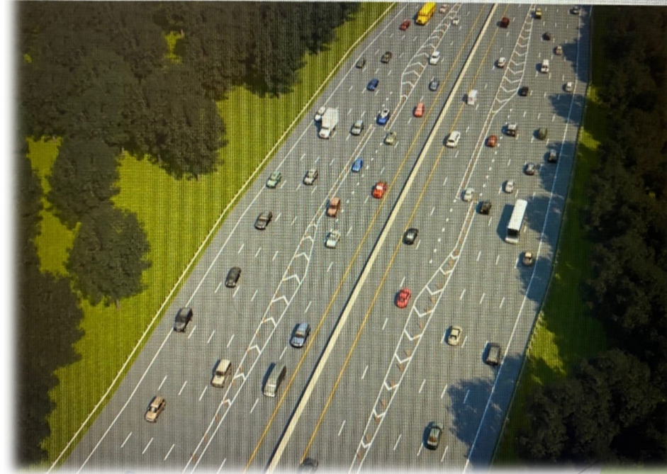
Figure 2-13: Example At-Grade Access Slip Ramp Configuration
