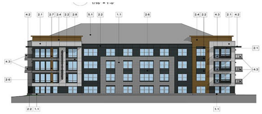
2 BUILDING 2000/3000 EAST ELEVATION 1/16" = 1'-0"
