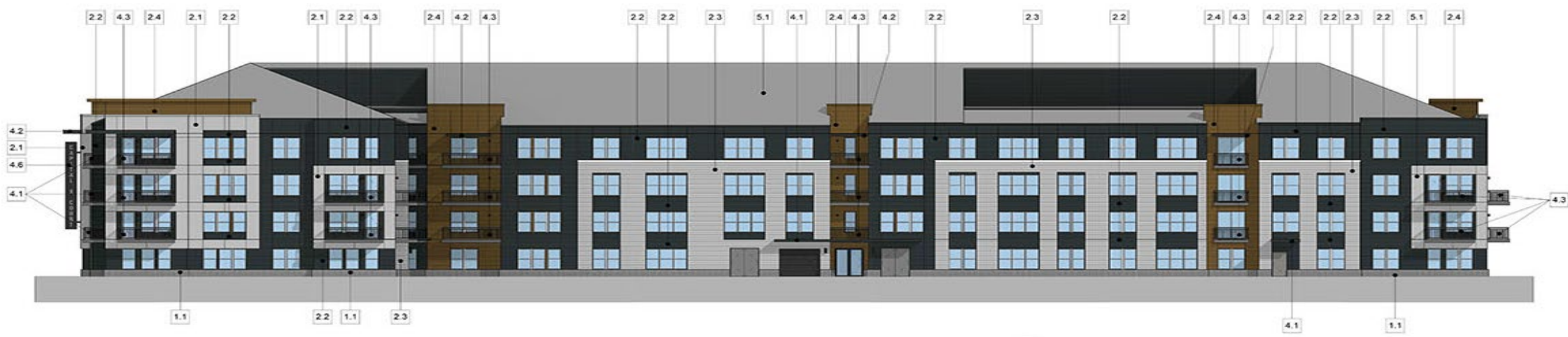
1 BUILDING 2000/3000 NORTH ELEVATION 1/16" = 1'-0"
