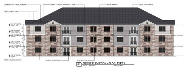
Figure 2: Typical Multifamily Building Elevation
