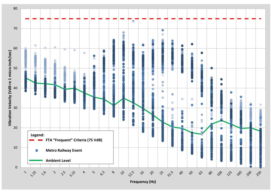
Figure 2: Maximum ground-borne vibration levels measured adjacent to railway.
