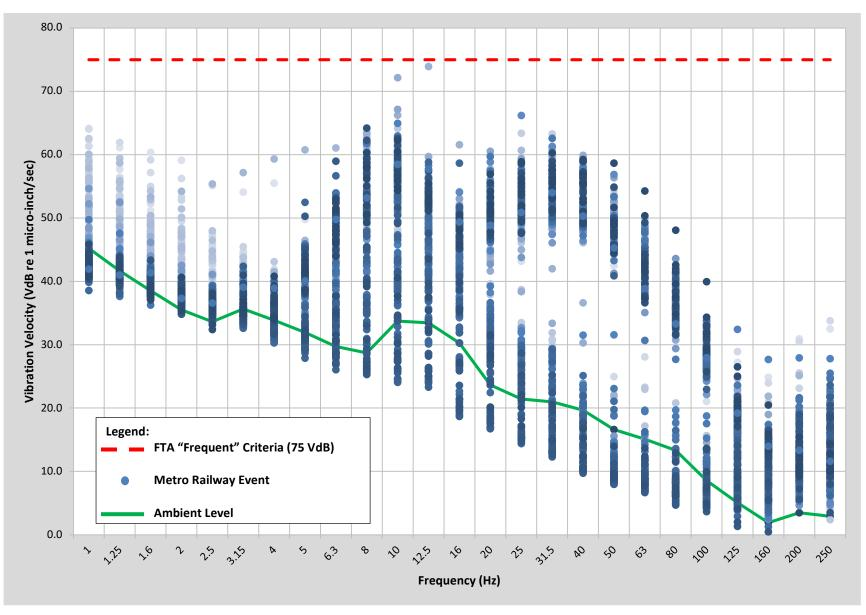
Figure 3: Maximum ground-borne vibration levels measured at nearest building location.
